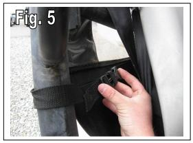
4. Remove the rear seat cushions for easy access to route the bottom straps around the seat mounting frame members. Route the passenger side bottom strap down below the outside seatbelt mounting bracket (fig. 6), across the seat frame members, down under the inside seatbelt mounting bracket (fig. 7) and up to the female buckle located in the bottom middle of the rear window (fig. 8). Repeat this process on the driver side.
